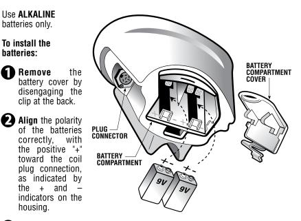
**B** Insert (2) 9-Volt ALKALINE batteries, with the contacts pointed inward, and press down on the back of the batteries to snap them into place.
